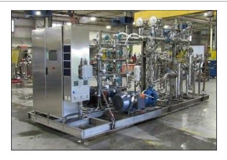
PRM constructed multiple custom stainless steel washing skids. Each was built on an open 304SS skid. The systems were integrated into a Siemens HMI PLC control platform to allow the operator complete control of the washing cycles. All components on each skid were either 304SS or 316SS and wired for Class 1 Div 2 hazardous locations.
